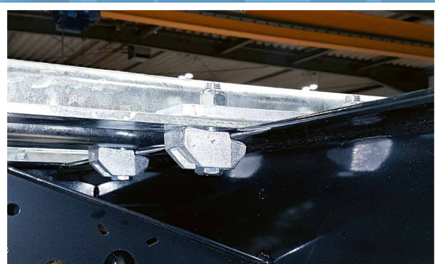
Sub frame secured using Type AF clamps
