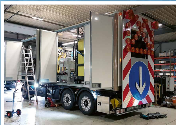
Diesel engine installed on trailer
