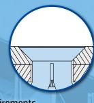
Hollo-Bolts also provided a clean architectural appearance, due to the flush fit head type, and excellent corrosion protection thanks to the zinc plated finish.
