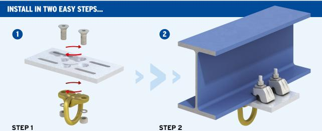
Fix the load ring in the orientation required with the supplied countersunk setscrews and anti-vibration washers then use a calibrated torque wrench to tighten to 100Nm.
